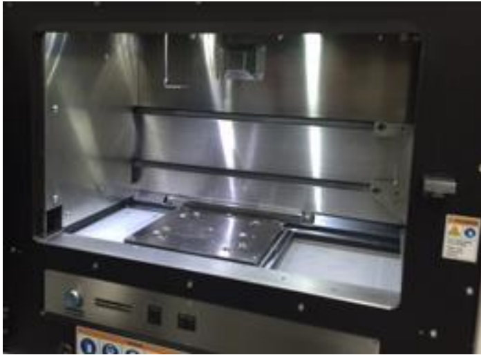
Typical Chamber in an AM Machine in a Laser Powder Bed Fusion Machine.
